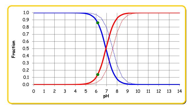
As can be seen from the graph, a solution of NaDCC with a pH of 6 to 7 has 80 to 90 percent of the active disinfectant in the form of HOCl, a solution of bleach with a pH of 11 to 12 has less than 10 percent of the active disinfectant in the more effective HOCl form. Essentially this means that NaDCC is far more effective as a disinfectant than bleach at much lower concentrations.
